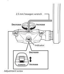
Do not turn the screw past the point at which the indicator shows the maximum or minimum tension.
